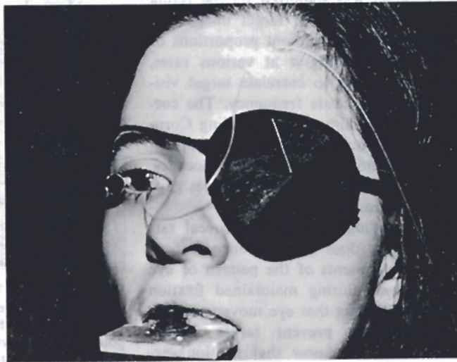
Fig. 2. (Left) A subject positioned for eye movement recording with a contact lens optical lever. The target (not shown) is located 2.04 meters in front of the subject's right eye. Head position is stabilized by a dental acrylic bite board. A narrow beam of collimated light, from the attenuated HeNe laser (0.15 milliwatt at the detector) on the right, falls on the flat front surface mirror which is attached by means of a stalk to a tightly fitting molded scleral contact lens held by suction (30 to 100 millimeters of mercury) on the subject's right eye. The mirror is oriented so that it is perpendicular to the line of sight, permitting horizontal and vertical rotations to be recorded free from confusion with torsions of the eye. The plane mirror also eliminates confusion of eye rotations with head translations. The laser light, after reflection from the contact lens mirror, falls on the surface of the photodetector shown mounted in Lucite on the left. The photodetector gives continuous two-dimensional indications of the position of the laser spot on the detector surface. (Right) Close-up view of the scleral contact lens during use. The flat front surface mirror is attached to the temporal side of the contact lens by means of a rigid aluminum stalk and self-supporting acrylic pedestal. The suction tubing, which is connected to the nasal side of the lens, can be seen taped to the subject's forehead as it passes to the suction apparatus (not shown).
