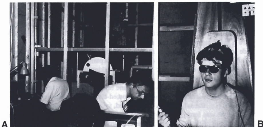
FIGURE 1.15. (A) Collewyn's large cube-surface field coil phase-detecting apparatus in Rotterdam. See the text for details. (B) Close-up of a subject in the apparatus shown in (A) wearing binocular eye coils beneath a pair of spectacles with a lowpass filter in front of one eye and a highpass filter in front of the other eye. These filters made it possible to present different stimuli to each eye, allowing psychophysical measurement of stereoacuity while head and eye movements were recorded.
