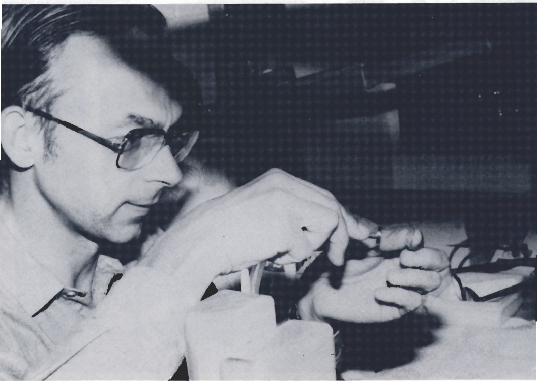
Fig. 2. Collewijn preparing a silicone annulus sensor coil (held with the thumb and forefinger of his left hand) prior to attachment to a human eye. His right hand holds a metal suction ring, which is used to hold the annulus as it is carried to the eye, where it is firmly pressed in place and adheres by the suction produced by its shape. The annulus weighs about 0.1 g and its twisted leads are very thin ( \sim 47\text{AVG} ).
