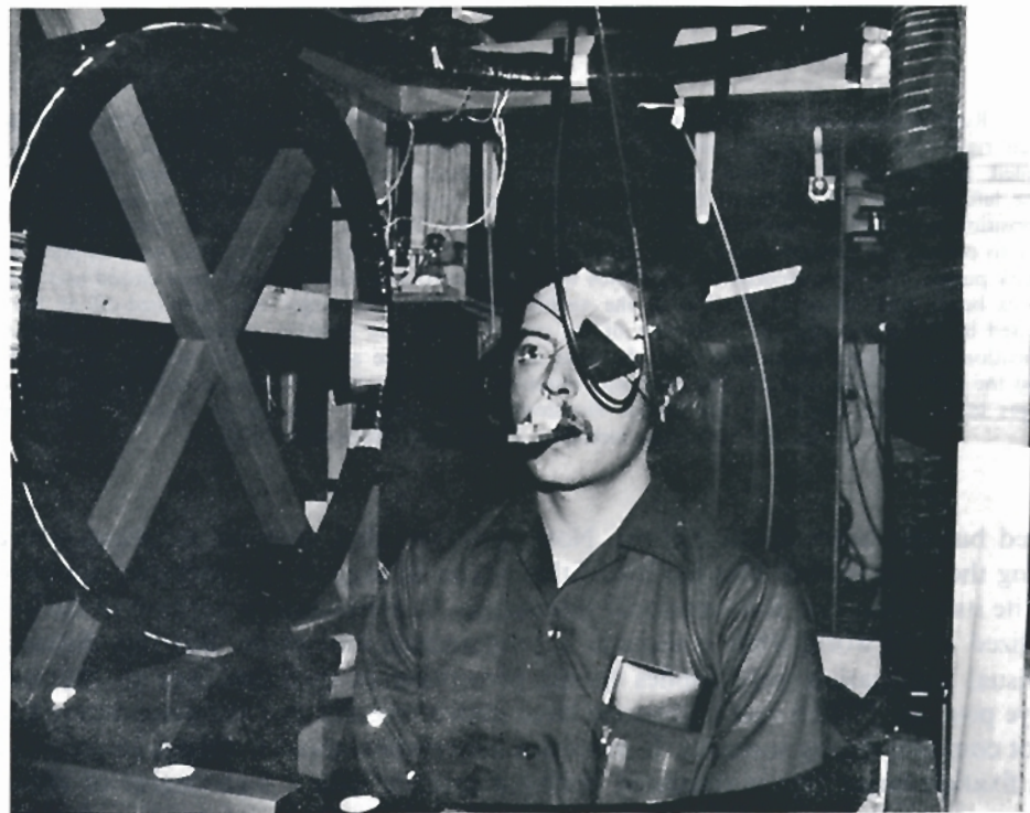
FIG. 11. Skavenski in position for simultaneous two-dimensional recording of rotations of his head and right eye by means of the magnetic field search coil technique. The eye search coil is embedded in a tight-fitting scleral contact lens held to the eye by suction. The head search coil is mounted to a dental bite plate. The field coils can be seen surrounding the subject who is looking at a target at optical infinity.
