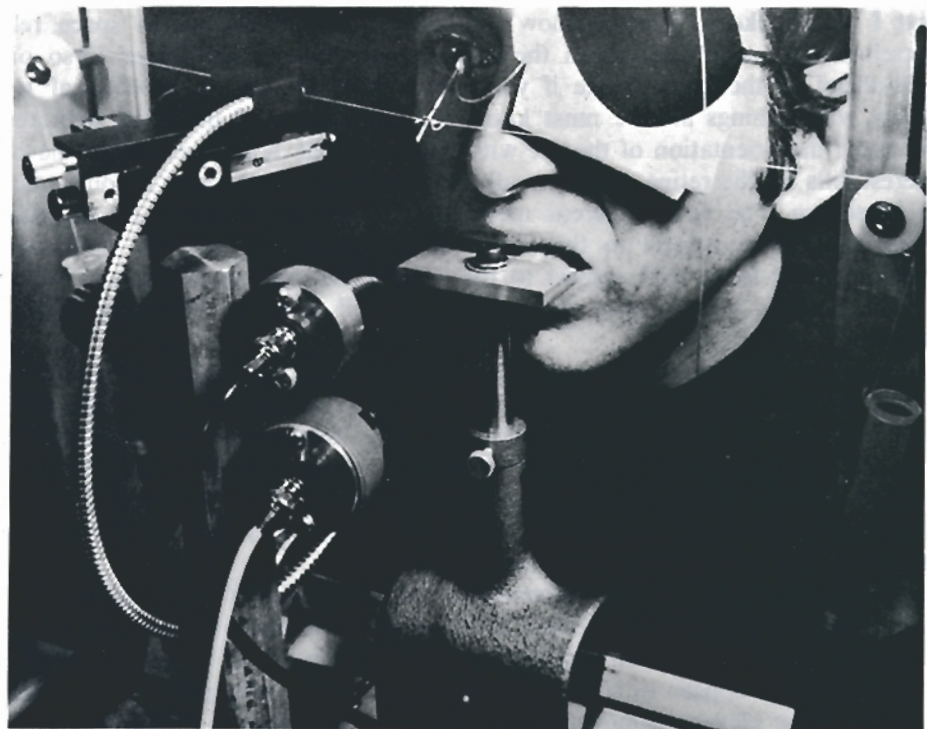
FIG. 9. Subject RS in position in the apparatus used to record horizontal eye movements while loading his right eye. RS is biting on an acrylic-bite board which holds his head rigidly in place. Horizontal rotations of his right eye were recorded by means of an infrared light transmitting and a collecting fiber optic mounted on the microscope stage just to his right. Loads were applied by adding water to the plastic chambers shown below the pulleys on the left and right. Loads were transmitted to the eye by means of the dacron threads that pass over the pulleys and connect to the 3-cm stalk attached to the scleral contact-lens. The contact-lens was held firmly to the eye by suction applied through the thin polyethylene tubing that can be seen as it passes up over the bridge of the nose and, again, as it passes in front of the left eye patch on its way to the suction apparatus (not shown). The suction tubing was arranged so that it did not, at any time during these experiments, touch the nose or face at any place except where it was taped to the forehead near the hairline. This contact with the skin could not have provided eye position information because the lateral displacement of the end of tubing at this junction with the contact-lens was too small and the tubing too flexible to produce any tactile cues on the forehead. With this apparatus loads of various magnitudes could be applied to the right eye gradually and completely silently. Taken from Skavenski (1972).
