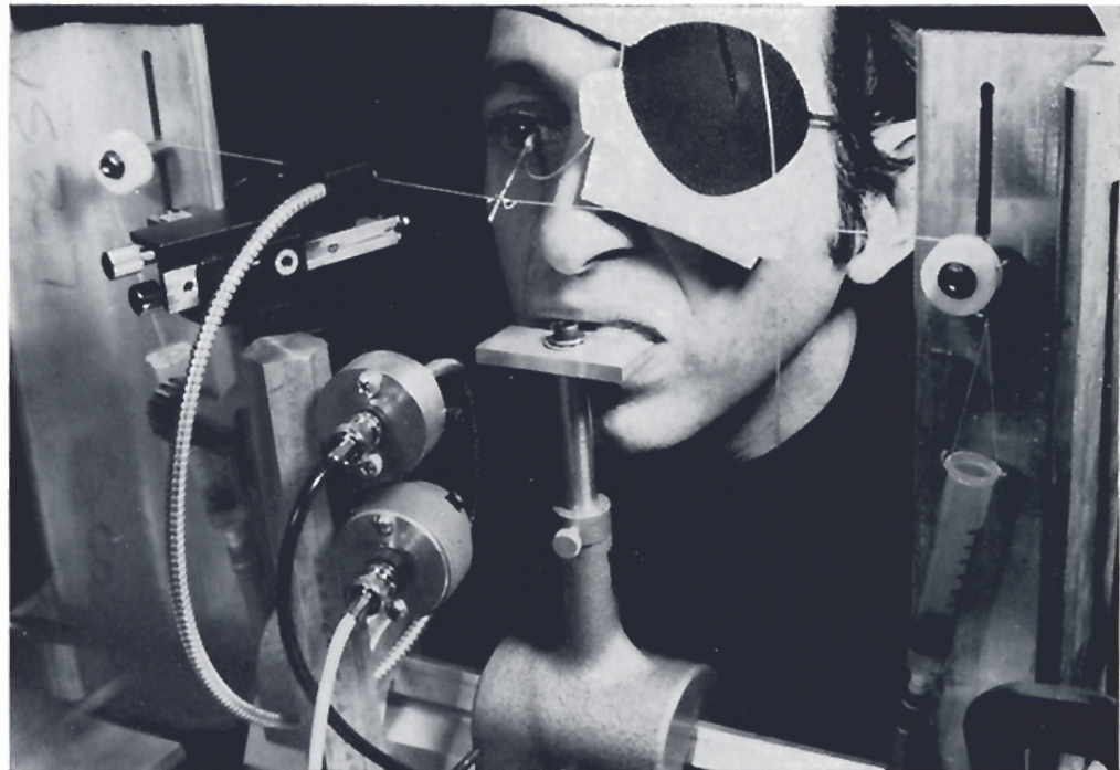
FIG. 1. Subject RS in position in the apparatus used to record horizontal eye movements while loading his right eye. RS is biting on an acrylic bite board which holds his head rigidly in place. Horizontal rotations of his right eye were recorded (for purposes described later in text) by means of an i.r. light transmitting and a collecting fiber optic mounted on the microscope stage just to his right. Loads were applied by adding water to the plastic chambers shown below the pulleys on the left and right. Loads were transmitted to the eye by means of the dacron threads that pass over the pulleys and connect to the 3 cm stalk attached to the scleral contact-lens. The contact-lens was held firmly to the eye by suction applied through the thin polyethylene tubing that can be seen as it passes up over the bridge of the nose and, again, as it passes in front of the left eye patch on its way to the suction apparatus (not shown). 4 With this apparatus loads of various magnitudes could be applied to the right eye gradually and completely silently.
